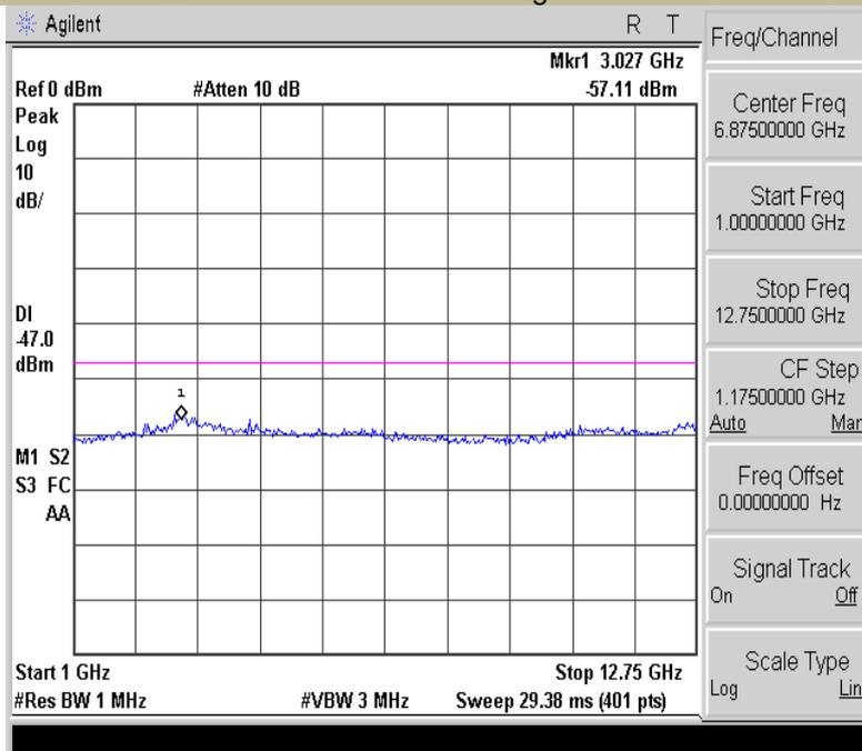
**Collateral Emissions of Receiver above 1GHz (30MHz to 1000MHz)**
