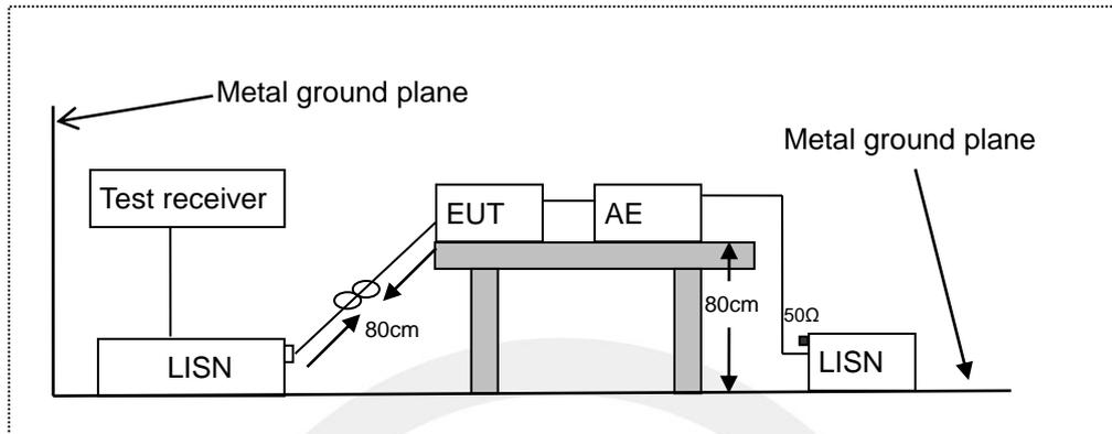
LISN: Line Impedance Stabilization Network
