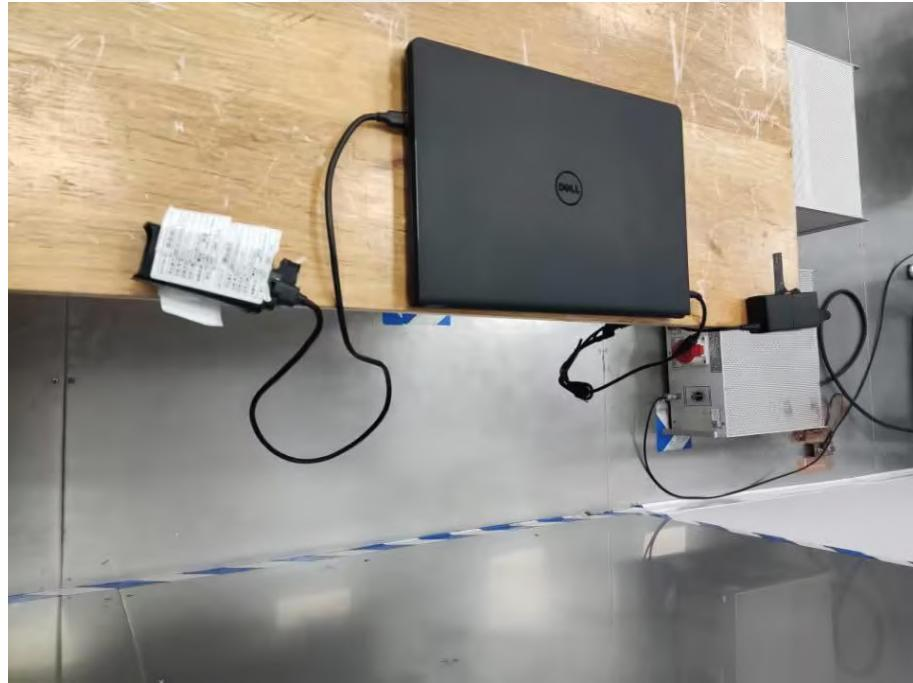
**17.2.Photo of Conducted Emissions at Telecommunications/network port Measurement**
