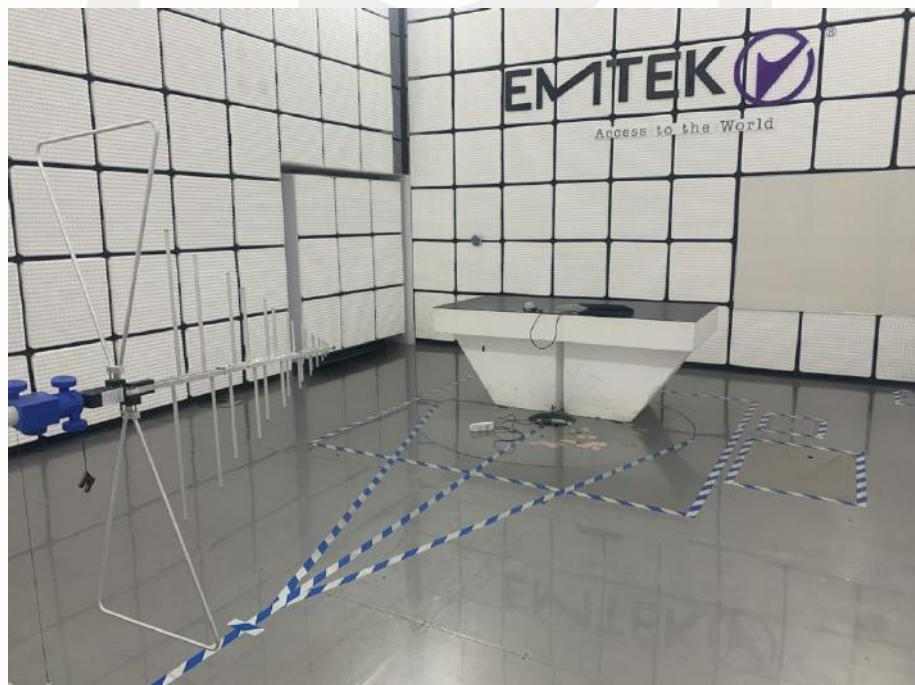
17.4.Photo of Radiation Emission Measurement ( Above 1GHz)
